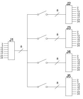
**NOTE:** Only switched "wires" are noted in the diagram above. All other pins can be configured as unswitched "through paths", or non-connected.
